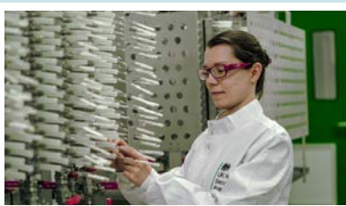
Fig. 1 – Freeze-dried glass ampoules loading onto the freeze-drier
